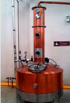
A tall, vertical industrial still made of copper. It has a large cylindrical base, a central column with several gauges and valves, and a smaller cylindrical section at the top. The entire unit is mounted on a metal base. | Máquina que a través de un proceso químico de ebullición, separa el alcohol de los demás componentes.                                                            |
