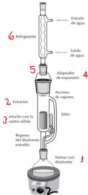
Figura 11: Partes del Extractor Soxhlet
