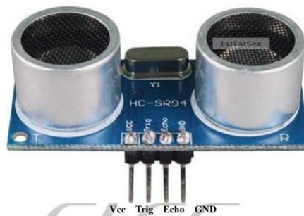
Figura 7. HC-SR04. Tomado de <http://www.electroschematics.com/wp-content/uploads/2013/07/HCSR04-datasheet-version-1.pdf>
