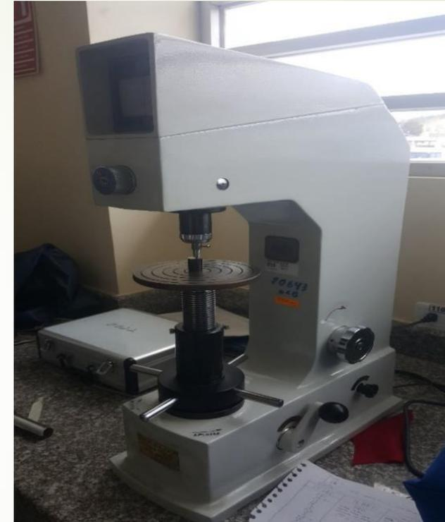
Norma utilizada: **ASTM E18**. *Standard Test Methods for Rockwell Hardness of Metallic Materials*
