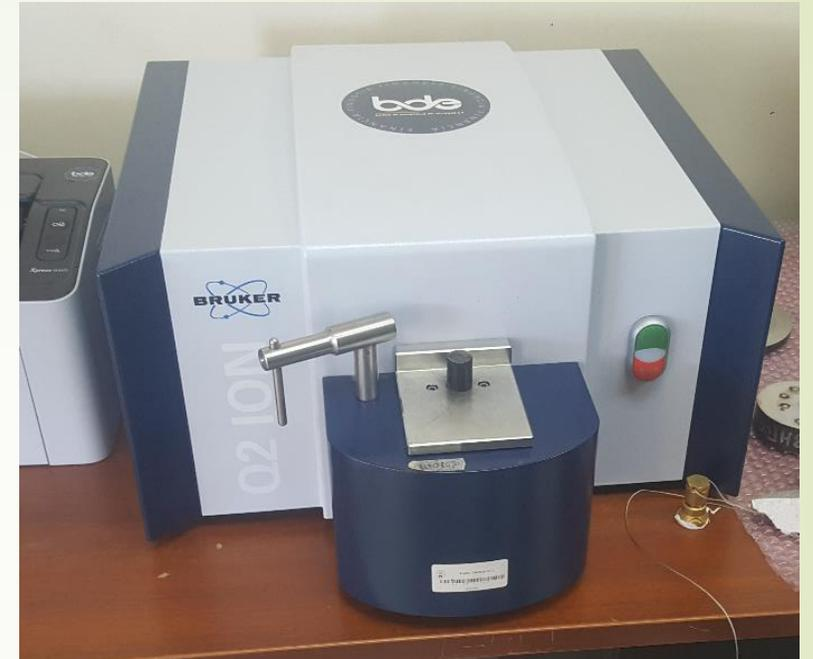
Norma utilizada: **ASTM E415**. *Standard Test Method for Analysis of Carbon and Low - Alloy Steel by Spark Atomic Emission Spectrometry.*
