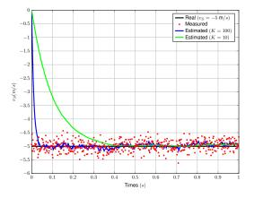
Figure 12: Slip velocity  $v_S$  estimation results with complementary filter.
