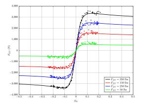
Figure 3: Pacejka Model vs. TTC Data for  $F_{ZT} = \{150, 250, 350\}$  lbs.
