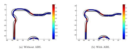
Figure 15: Brake plot over a typical FS lap.
