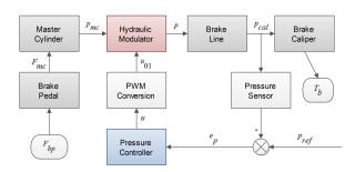
Figure 5: Schematic of brakeline dynamics and pressure controller.
