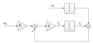
Figure 11: Block diagram of complementary filter.
