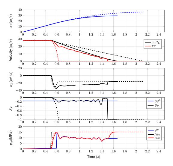
Figure 13: Comparative simulation results with (solid) and without (dashed) ABS.
