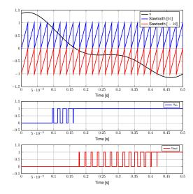
Figure 6: PWM implementation with  $f_c = 50$  Hz.
