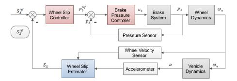
Figure 4: Proposed control structure.
