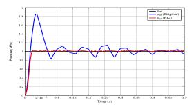
Figure 7: Step response with PD controller for  $p_{cal}$ .
