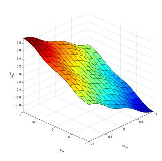
Figure 10: Output surfaces of FIS models for wheel slip controller.
