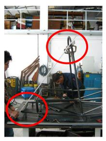
Figure 15 The angle of the main hoop bracing
