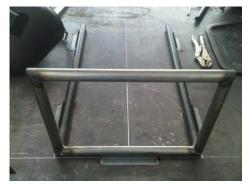
Figure 10 Front bulkhead welded to the floor
