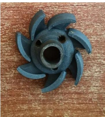
A photograph of the same blue impeller as in the previous images, resting on a wooden surface. The blades are noticeably bent and deformed, with a loss of their original curved shape. |
