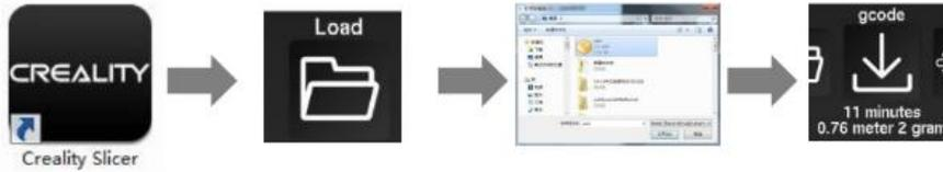
Open the software→Load→Select the file→Wait for slicing to finish ,and save the gcode file to TF card.
