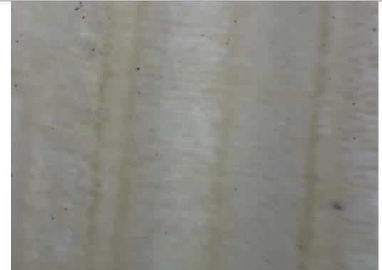
Probeta PVA a 210°C
