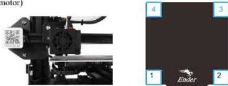
3. Move the nozzle the front/left leveling screw and adjust the platform height by turning the knob underneath. Use a piece of A4 paper (standard printer paper) to assist with the adjustment, making sure that the nozzle lightly scratches the paper.
