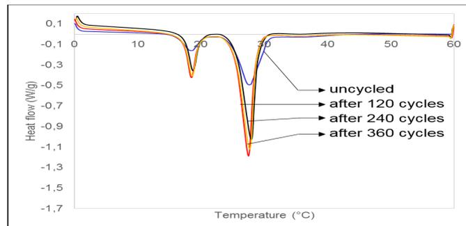
**Figure 2.** DSC melting curves of PCM supported in calcined diatomite before and after the application of 0, 120, 240 and 360 thermal cycles using 100% commercial stearic acid esters
