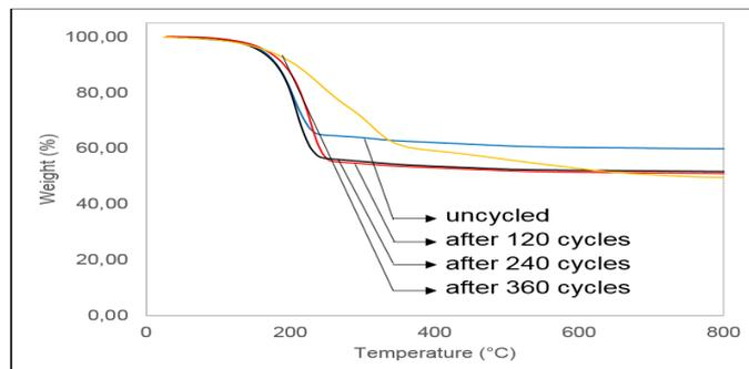
**Figure 3.** Thermogram of the PCM supported in calcined diatomite before and after the application of 0, 120, 240 and 360 thermal cycles, using 100% commercial stearic acid esters
