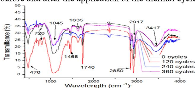
**Figure 4.** FT-IR spectra of the PCM supported in calcined diatomite before and after the application of 0, 120, 240 and 360 thermal cycles using 100% commercial stearic acid esters
