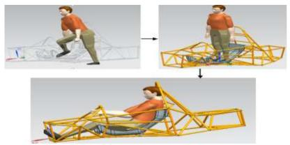
Fig.11. Select the 1% percentile human body model to simulate in and out of the cabin
