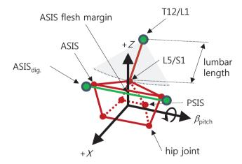
Fig. 5. The three dimensional coordinate system to translate and rotate the pelvis geometry.
