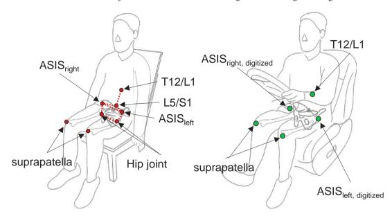
Fig. 4. Illustration of digitized body landmarks, estimated joint locations, and pelvis bony landmarks in the hardseat (left) and the vehicle seat (right), respectively. The dotted line in the left image shows pelvis-lumbar segments.
