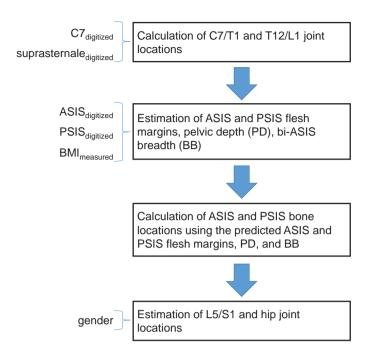
Fig. 2. Estimation procedure for a driver's inner joint and pelvis bony landmark locations using hardseatdata [2, 13].
