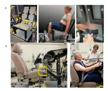
Fig 1.Constructed hardseat and driver mockup to measure body surface landmark locations.(a) hardseatand recording a participant's posterior-superior iliac spines (PSIS) landmark location; (b) driver mockupand recording body landmark locations using a FARO Arm coordinate digitizer.
