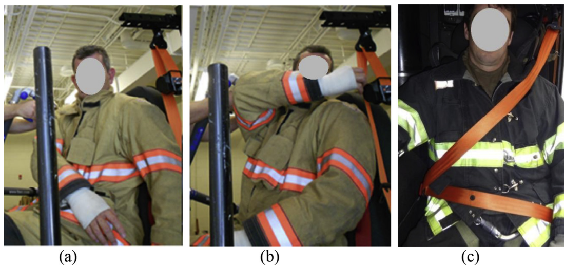
Fig. 7. (a) A fire apparatus simulation buck was used to measure the lap belt length (Type I belt) and 3-point belt length (Type II belt). (b) A test of maneuvering seat belt. (c) Measured belt lengths, including the length to seatbelt anchor points and the additional slack required to span both lap belt and shoulder belt.
