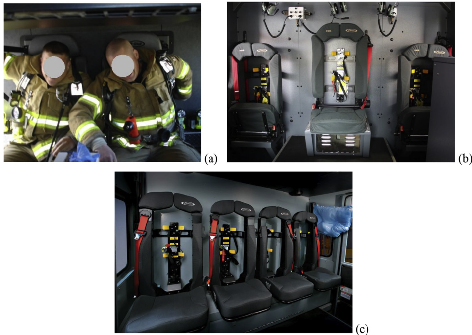
Fig. 6. (a) The challenge is apparent for two firefighters to sit in a row with current space specification of 560 mm for each person as seen in the fire truck with two forward-facing crew seats along the rear wall. (b and c) Three and four forward-facing seats in a row along the rear wall are seen in current fire trucks. Changing the unit space from 560 mm to 733 mm would afford three seats in a row with an acceptable unit space for each, which is a practical and cost-reasonable solution for seats along the rear wall.
