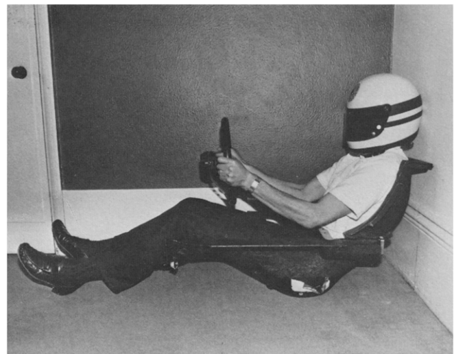
Fig. 2 Driver in-situ in the seat showing angles of backrest, neck, arms and legs
