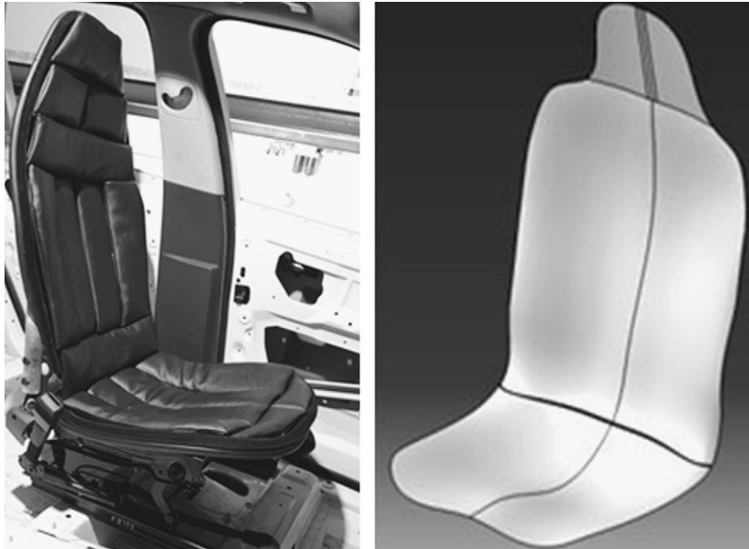
Fig. 1. New car-seat concept based on the human body contour developed at BMW (Franz et al., submitted for publication).
