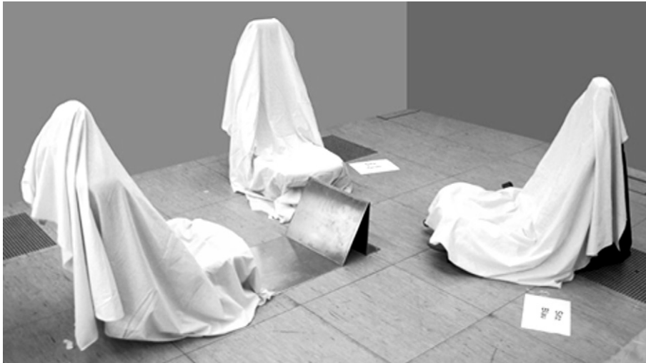
Fig. 3. Research set-up with covered seats. The seats are deliberately covered so participants are not influenced by the appearance of the seats and focus on the seats' sitting comfort.
