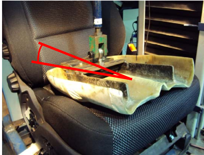
Figure 1 Positioning of an indenter form relative to seat at 10 deg. from horizontal (see online version for colours)
