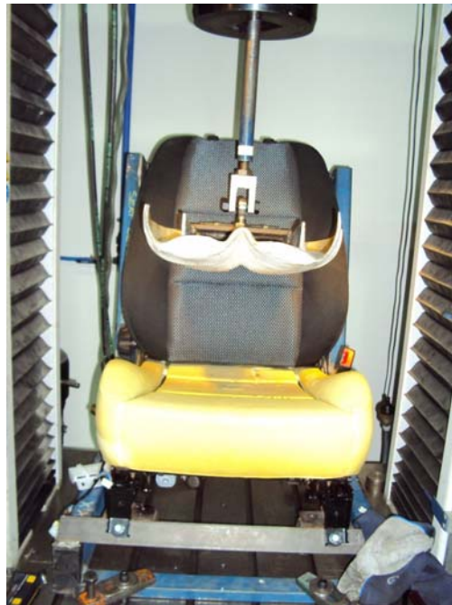
Figure 2 Indentation on seat with trim removed (see online version for colours)
