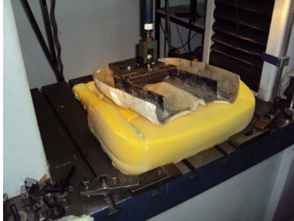
Figure 4 Indentation on foam pad only (no seat) (see online version for colours)
