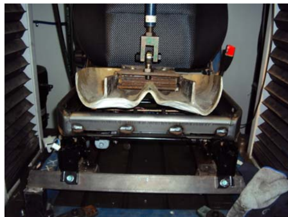
Figure 3 Indentation on seat suspension with foam and trim removed (see online version for colours)
