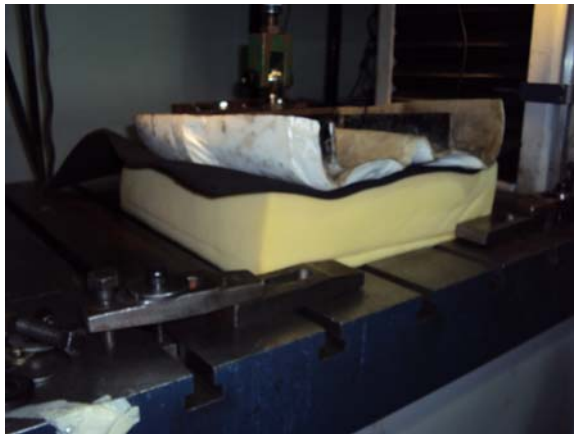
Figure 5 Indentation on foam pad with intermediate neoprene layer (no seat) (see online version for colours)
