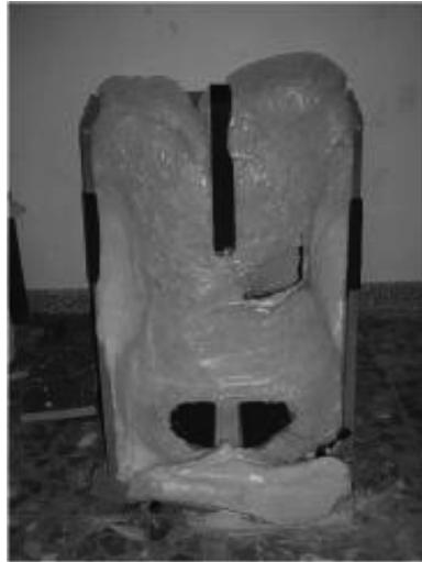
Figure 21 Polyurethane mould obtained from the driver's back and buttocks
