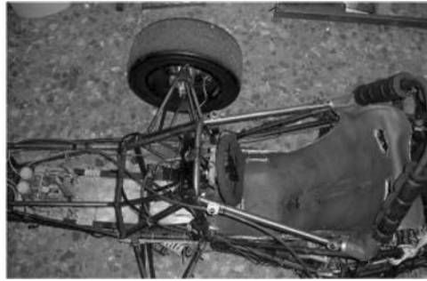
Figure 19 End result of the single-seater cockpit with all the controls
