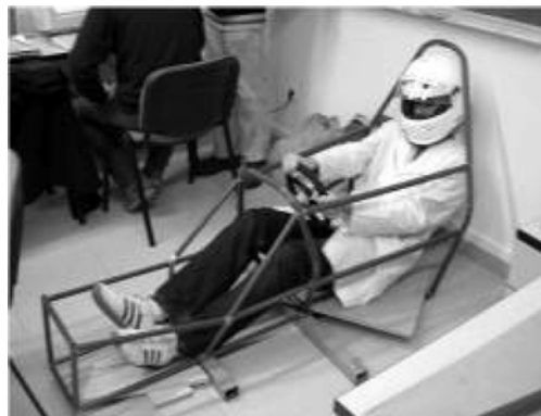
Figure 18 Model of the PVC chassis tested by a 98% percentile driver
