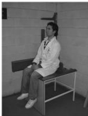
Figure 5 Anthropometric measuring table
