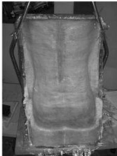
Figure 22 Fibre glass seat on the mould
