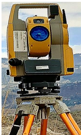
Figura 10 Estación Total topcon series direct aiming station
