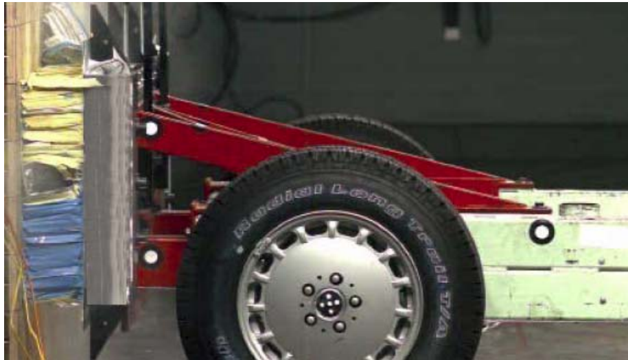
Figure 1.6 – AE-MDB condition B final deformation
